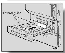
4 Load the paper into the drawer so that the side of the paper to be printed on (the side facing up when the package was unwrapped) faces up.
